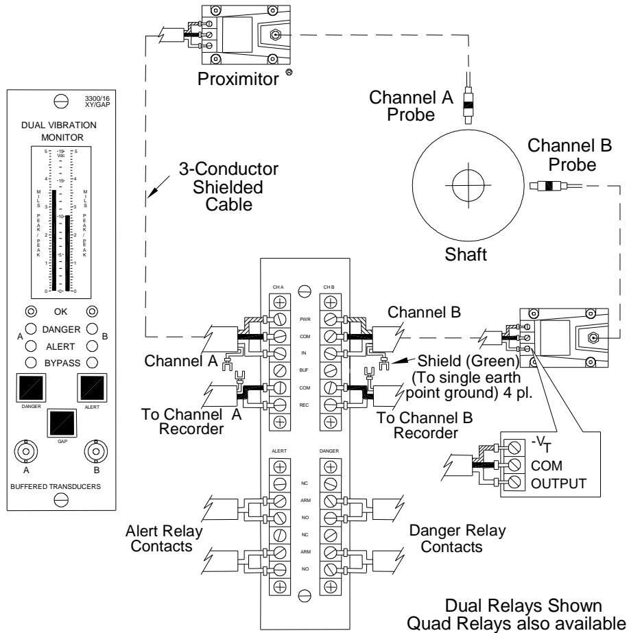
Field wiring diagram for 3300/16 XY/GAP Dual Vibration Monitor
